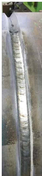
Pipe welding(3G) (170A/27V)
