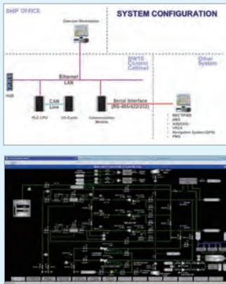
HiBallast Human Machine Interface (HMI) is easily expandable, helps easy operation, and enables to be flexibly integrated such as:
