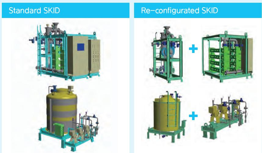
Space and transportation of equipment would be challenges for BWTS retrofitting. HiBallast skid can be divided into several units considering installation space and hatch size.
