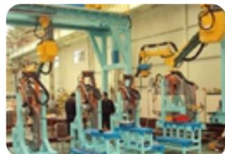
GANTRY WELDING MACHINE FOR RAILWAY CAR ASSEMBLY
