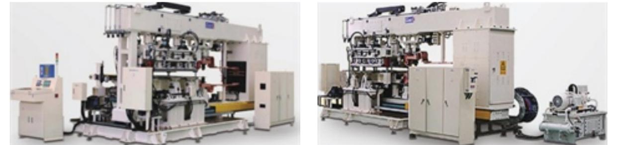
Mash seam welders are used by steel manufacturers for connecting coil in many different processes, including Continuous Galvanizing Lines (CGLs), Annealing & Coating Lines (ACLs), Multi Coating Lines (MCLs), and Continuous Annealing Lines (CALs). 50 to 100 units are typically used in the iron making process. The acid treatment line (CPL) below is a schematic diagram as an example.
